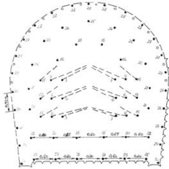
Fig. 3a: Positioning of the blasting holes for very hard types of rocks
